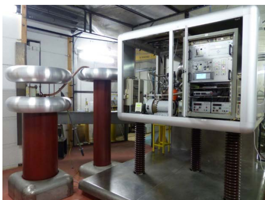
Figure 1: The HV head of the GENEPI2 accelerator (left) and the experimental area of the GENESIS platform with the XY table in front of the target foreground (right).
