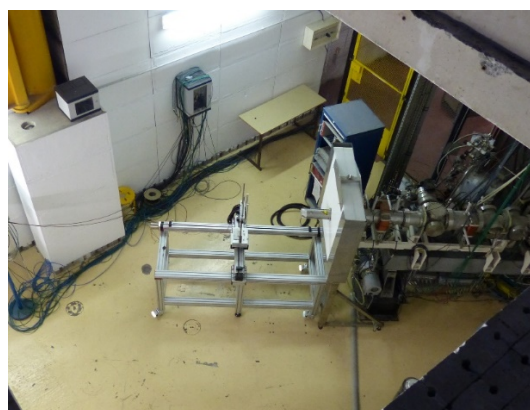
Figure 1: The HV head of the GENEPI2 accelerator (left) and the experimental area of the GENESIS platform with the XY table in front of the target foreground (right).
