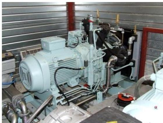
Three stages room temperature helium gas compressor
