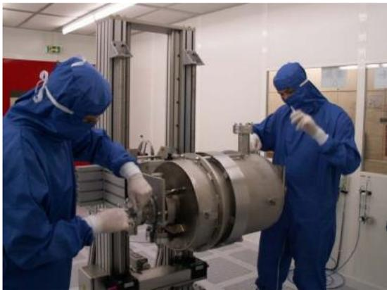
Assembling of cavity for power coupler conditioning
