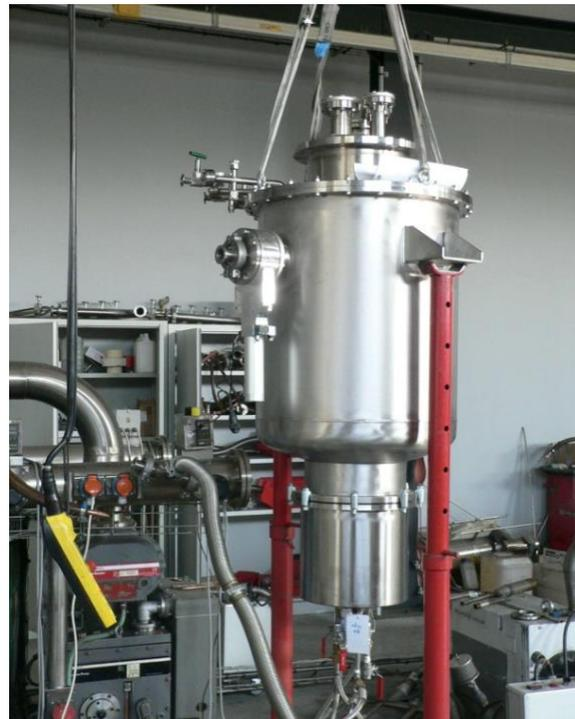
Helium refrigerator and one cold box of spiral2 superconducting linac
