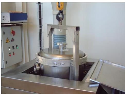
Ultrasonic cleanin: 200L Ultrasonic bath operating at a power of 10 kW/l
