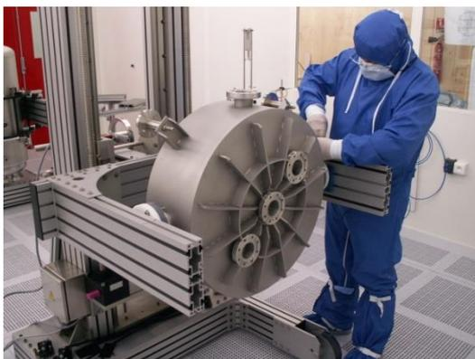
Assembling of 700 MHz protons cavity (R&D for MYRRHA)
