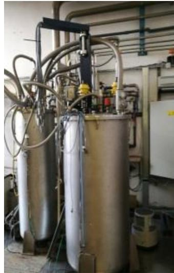
Cryostat and calibration cryogenic insert
