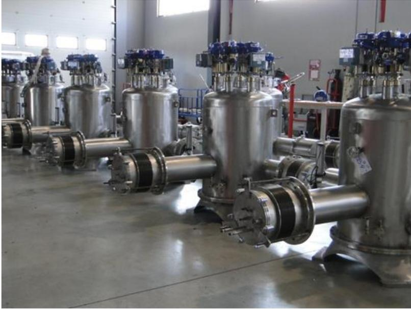
Cold boxes of spiral2 superconducting linac
