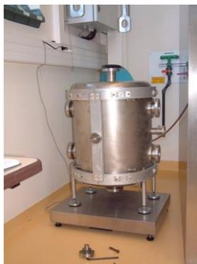
Weighing of a cavity
