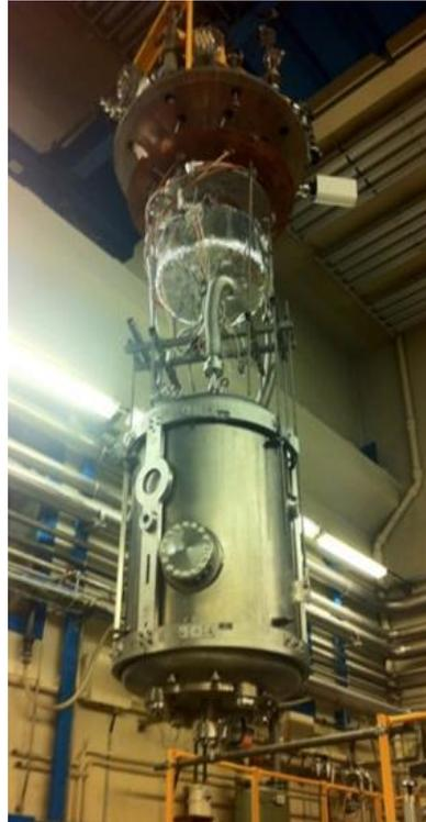
Vertical test of cavities of a ESS double spoke cavity (f=352 MHz)
