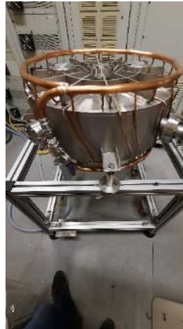
Cavity for the RF conditioning of the couplers
