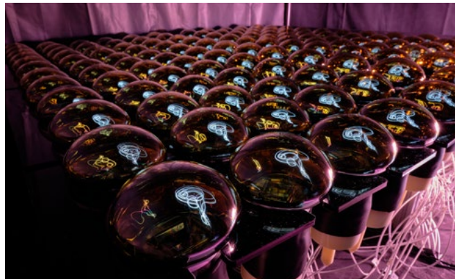
Test device for the electronic signal digitisation system associated with the photomultipliers of the JUNO detector by LP2i Bordeaux. © Jean Jouve
